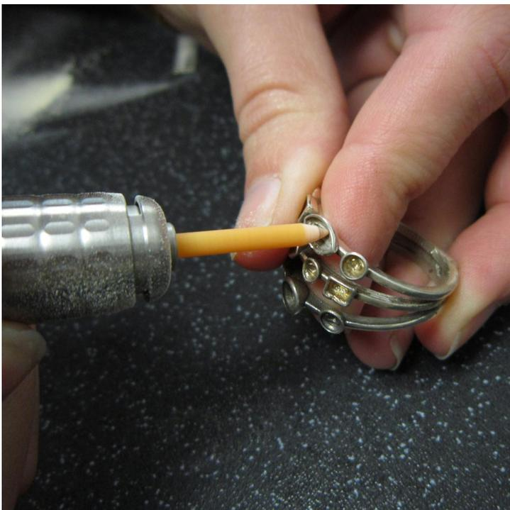
Using a 2.35, 3.00 and even 1.6mm Diameter Ceramic stone they can be fitted directly into the collet on the Rotary handpiece.
